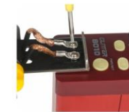
3. Tighten the screws. (Keep copper wires separate)
