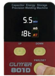
5. Press the power and the "▲/▼" buttons to change your spot welding mode, such as AT/MT switch.
