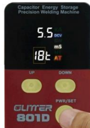
4. Set energy grade— To customize the energy grade, you need to press the power button when the machine is on. The current number will flash, you can adjust the number through "▲/▼" buttons.
