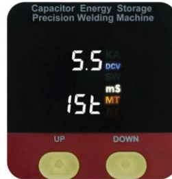
3. When the voltage is between 5.2 and 5.8V, the machine is ready for use.
