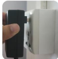
② Plug the adapter into an AC 100-240 volt wall socket to charge the machine.
