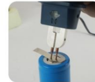
2. Hold the welding pen and apply a certain pressure to the object's surface (e.g. nickel strip) simultaneously. Automatic welding begins after about 20ms.
