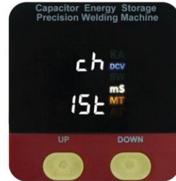
2. After the machine is powered on for the first time, the LED will show "CH" intermittently and the real-time voltage value of the internal capacitor. The spot welder is being charged.
