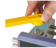
1. Insert the welding head into the corresponding socket.
