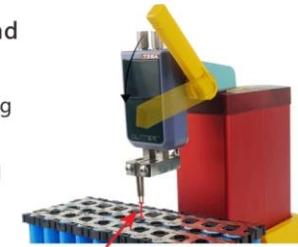
The distance between of the welding needle and battery is 4-9mm.
