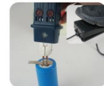
3. Hold the welding pen and apply a certain pressure to the object's surface (e.g. nickel strip) simultaneously. Release energy by controlling the foot pedal.
