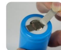
3. Check the spots' reliability. Finish spot welding.
