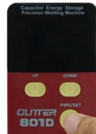
6. When the machine is not in use, please press and hold the power button for 2 seconds and unplug the power adapter from the wall socket.
