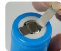
4. Check the spots' reliability. Finish spot welding.
